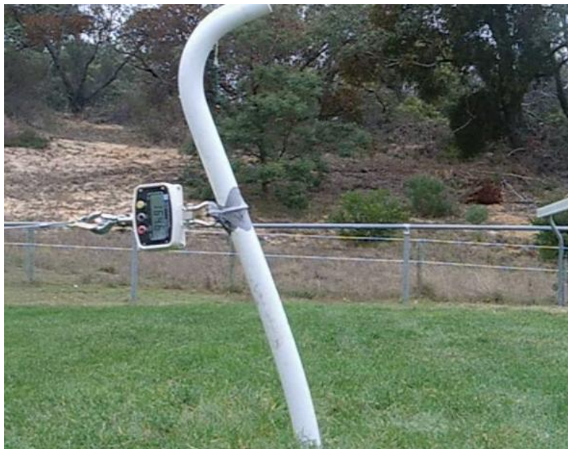
Figure 2: Test type B was conducted using an instrumented winch attached to the post 700mm from the ground. These tests are useful for characterising the force deflection characteristics of the post and determining the pseudo static cantilever breaking load for any fuses. In the figure, a new style of footing is being trailed. The post was able to manage the loading. The footing turned in the ground at 164.6 kg as seen on the crane scales in the figure.
