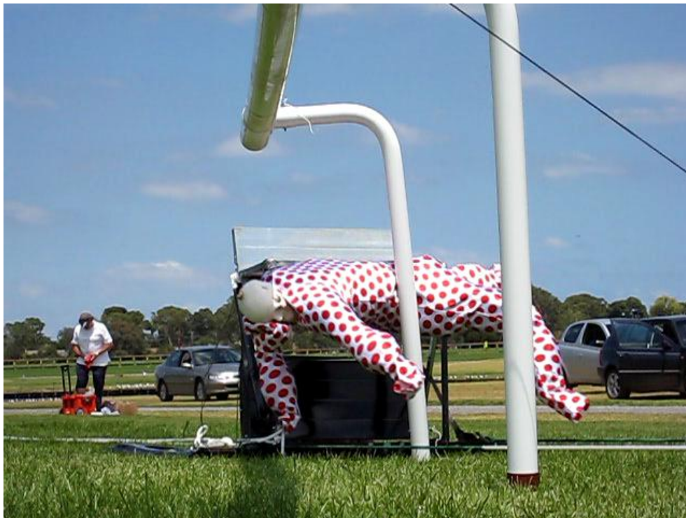
Figure 3: Type D testing, a ballast dummy is projected into contact with the post. Type C was similar in that a ballast dummy was also used, but the dummy was released in a head on-impact configuration with the post.
